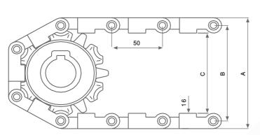
Belt surface: Open belt with a smooth surface. Open area: 27%. Biggest opening 5 x 9 mm. Strength: The right belt for heavy applications. Material: PE, PP, POM. Oclour: nat/white, grey/blue.
